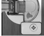
Note: To reset the Soft-close damper, move the adjustment switch to "Strong", then to the desired position. Close the door and the Soft-close will be reset.
