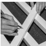
**STEP 13** - Drill a 5/8" hole through **ONE** side of picket, not both.
