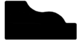
Shingle Mould - 8 ft D210 - 7/8" x 1-5/8"
